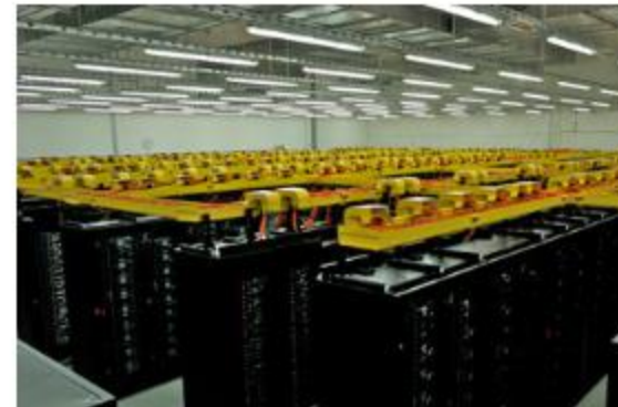
SuperMUC uses 40 percent less energy than would be required by an equivalent air-cooled system.
